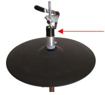
Now install your new drop clutch on the Hi-Hat stand. Make sure the latch portion of the drop clutch resides at the top of the black channel. It must be inside the groove of the black tube. We suggest that the top of the latch is even with the top of the black channel like the illustration. Now tighten the large butterfly bolt on the drop clutch to lock it in position on the Hi-Hat stand.
